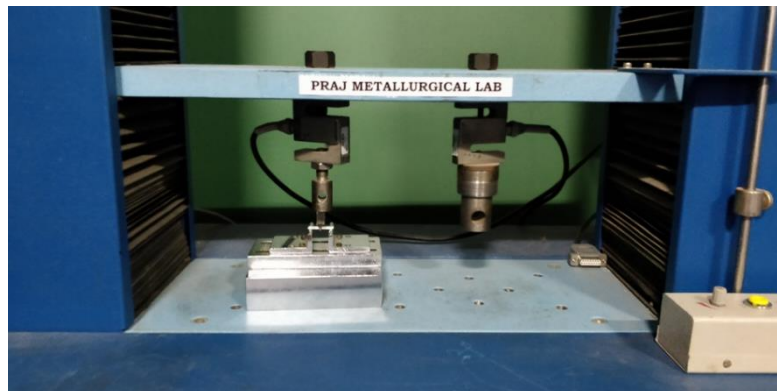
IMAGE 3B :UNIVERSAL TESTING MACHINE FOR FLEXURAL STRENGTH
